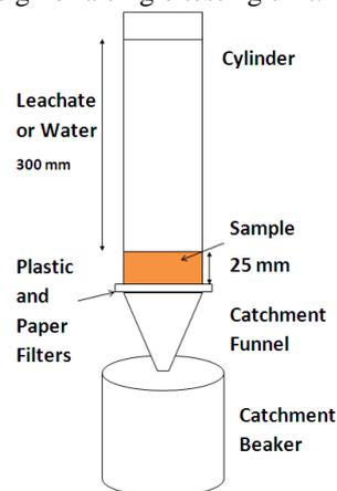
Figure 1 – Long Term Test Design
