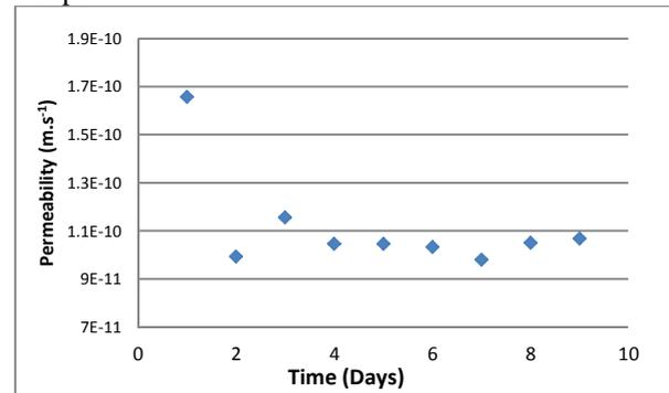
**Figure 6 – Clay sample, daily permeability readings**
