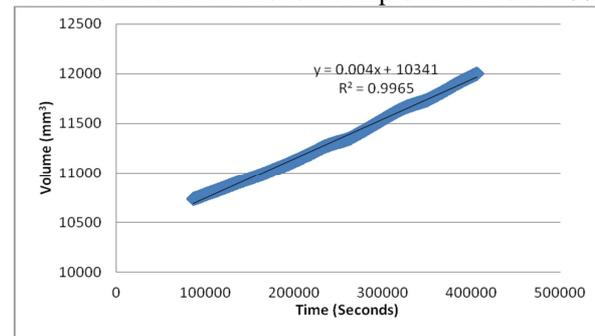
**Figure 7 – Polycom Sample, Volume vs. Time**
