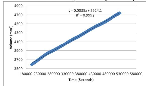
**Figure 5 –Clay Sample, Volume vs. Time**
