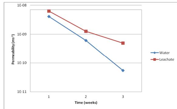
Figure 9 – Permeability of clay sample, water and leachate permeation over three weeks.
