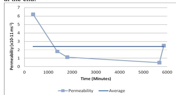
**Figure 2 – Golder permeability of Clay sample.**
