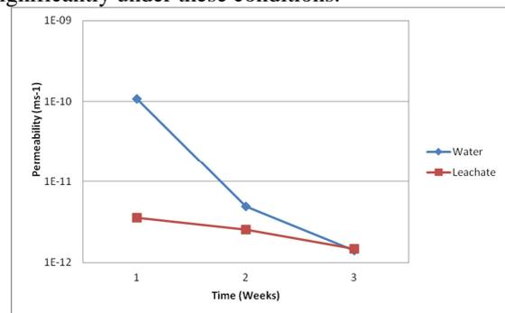
Figure 10 – Permeability of the Polycom sample, water and leachate permeation over three weeks.
